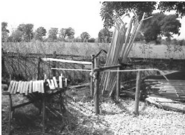
A roof rib (bent on the extreme right) on a shaving post.
