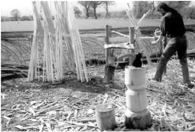
Shaving the wall laths on the shaving post.
